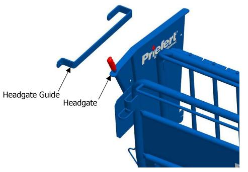
**Step 8:** Insert the 5/8"x3½" bolt and washer into the Headgate and secure it to the **(CT)** Floor.
