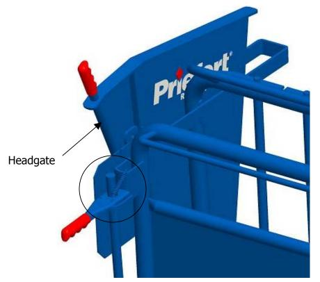
**Step 10:** Insert the Latch Handle into the Trigger Box and attach the spring.
