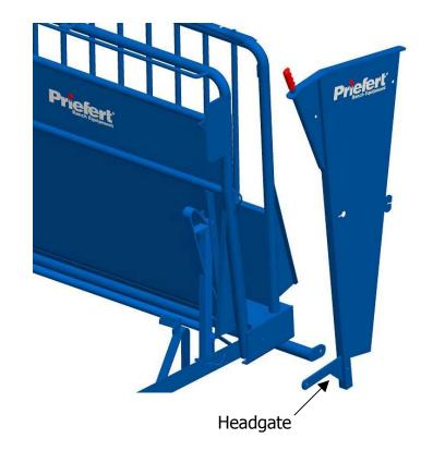
**Step 6:** Remove the 5/8"x3½" bolt and Washer attaching the Headgate to the **(CT)** Floor.
