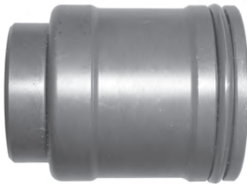
Fig. 6 - Small end of Hammer is toward the anvil.
