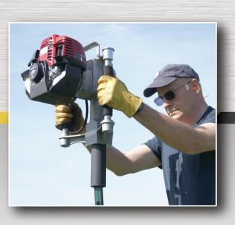
The driver is manufactured from the very best materials to promote long tool life, including heat-treated alloy steel, "aircraft quality" aluminum, stainless steel fasteners and bearings on all rotating parts.
