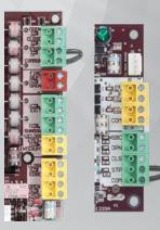
Includes 3 Monitored Safety Inputs to cover all entrapment points. (Add 3 more inputs with optional Expansion Board).
