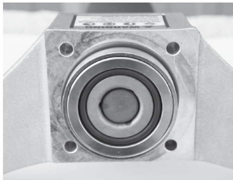
Fig. 12 - View when Lower Driver Body removed.
