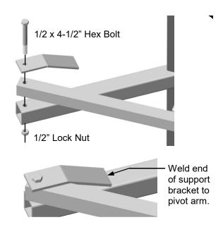
Mount the primary LGK arm and gate arm to the secondary arm as shown. Actuator should be extended.
