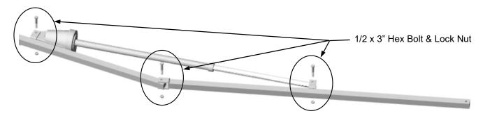
Align the end of the primary LGK arm to the gate and mount the gate bracket. Limits may now be adjusted as per the from gate arm manufacture installation manual.
