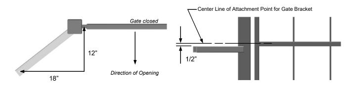
Pivot arm must be level for proper operation.
