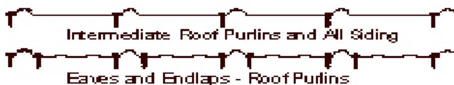
Shown above are the fastening patterns recommended for the proper installation of the metal panels.
