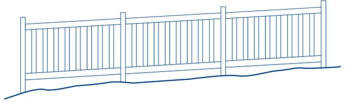
When installing multiple sections, it is advisable to use an End Post and field fabricate the opposite side of the post to avoid a jagged fence line.
